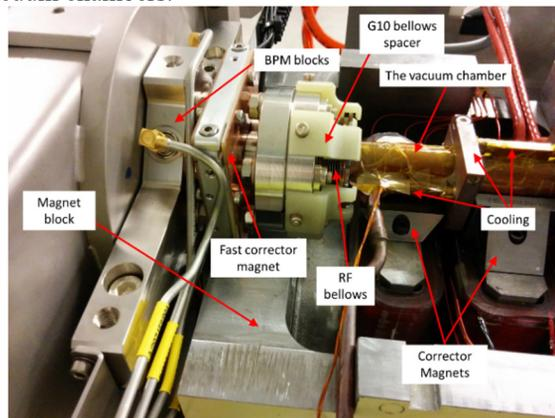
Figure 2: Location of BPM block and bellows.
