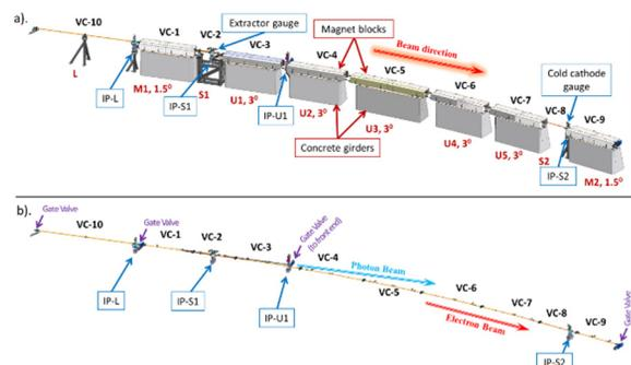
Figure 1: One standard 3 GeV storage ring achromat, a). with the magnet blocks and girders b). the vacuum chambers without the magnet blocks [3].
