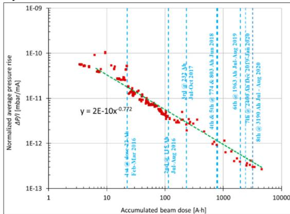
Figure 3: 3 GeV ring: normalized average pressure rise  $\Delta P_{av}/I$  [mbar/mA] vs. beam dose [Ah].
