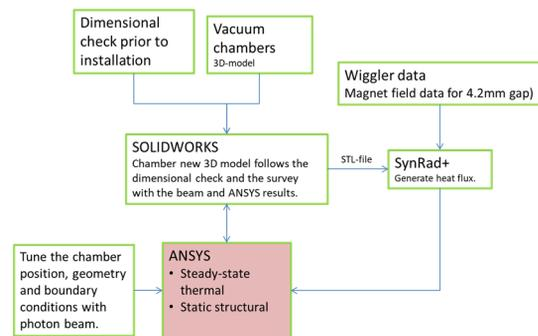
Figure 5: Workflow used to investigate hot spots and validate machine operational conditions.
