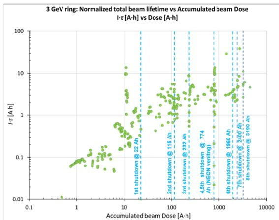
Figure 4: 3 GeV ring: normalized beam lifetime  $I\tau$  [A·h] vs. beam dose [Ah] [3].
