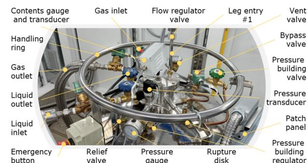
Figure 2: Top of primary LN2 cylinder and description of the connected elements.
