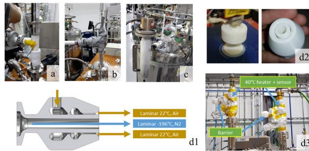
Figure 6: Options against condensate formation: nothing (a), blanket with heaters (b), gas heater (c), and custom part with air barrier (d).
