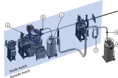
Figure 1: Third optical hutch of the CARNAÚBA beamline, highlighting the liquid nitrogen supply system of the 4CM, which comprises the vacuum chamber (a), the cryostat (b), the primary (c) and secondary (e) LN2 cylinders, the transfer line (d) and the exhaust line (f).
