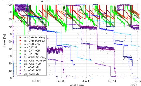
Figure 3: Levels of primary and secondary LN2 cylinders of CARNAÚBA and CATERETÊ beamlines.
