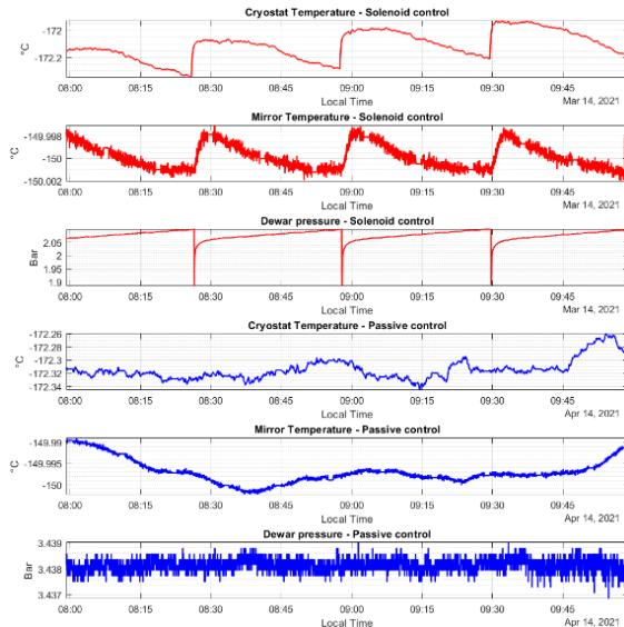
Figure 4: Temperature and vessel pressure when using the active solenoid control or the passive valve at the CNB:M1 systems.
