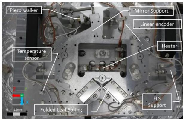
Figure 1: Fully assembled CAT M2 internal mechanism.
