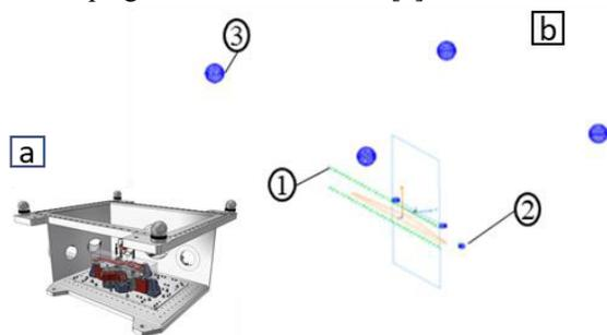
Figure 2: (a) CAT M2 CAD representation and (b) CAT M2 internal mechanism fiducialization measurements: (1) mirror optical face, (2) mirror internal mechanism, and (3) fiducialization points.
