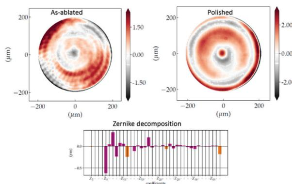
Figure 3: Top: Left: a typical figure error of as-ablated lens. Right: figure error of the polished lens. Bottom: Figure error decomposition into Zernike polynomials.
