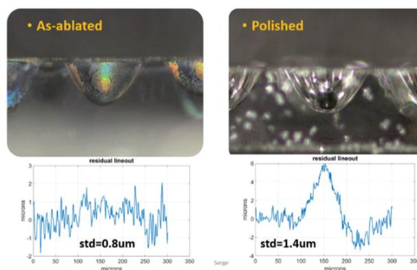
Figure 1: Top: Optical image through a polished side of the diamond plate. Left: as-ablated lens. Right: Polished lens. Bottom: corresponding lineouts of paraboloid fit residuals.
