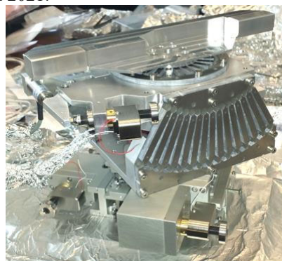
Figure 6: A photograph of the pilot nanositioning stages for CBXFEL diamond crystal manipulation.
