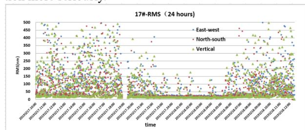
Figure 6: RMS value of 24-hour vibration.
