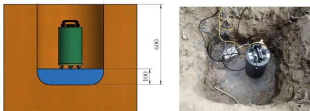
Figure 2: Installation method of seismograph.
