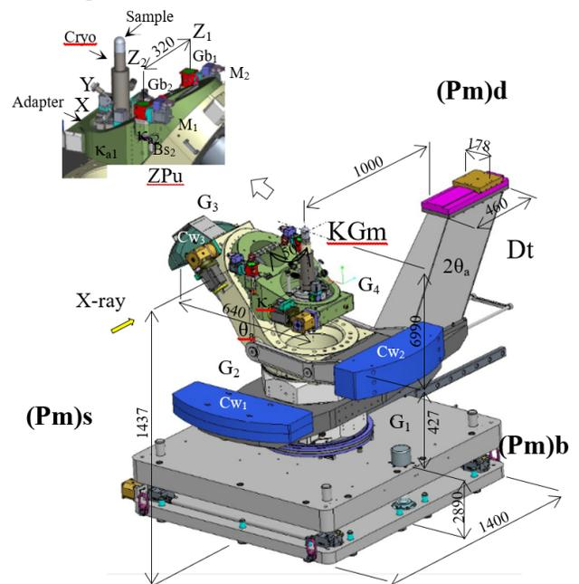
The whole device is being carried by a precision (G440/X2W2) gonio for which a compact solution has been applied for its static balance (CW2-counterweight). On top (and, inside) of the last gonio, a cryostat (CS202SK) is being held through a dedicated interface. It is a relatively simple (reliable) and efficient (economical) instrument for low temperatures (4.2K ÷325K) experiments [10].
