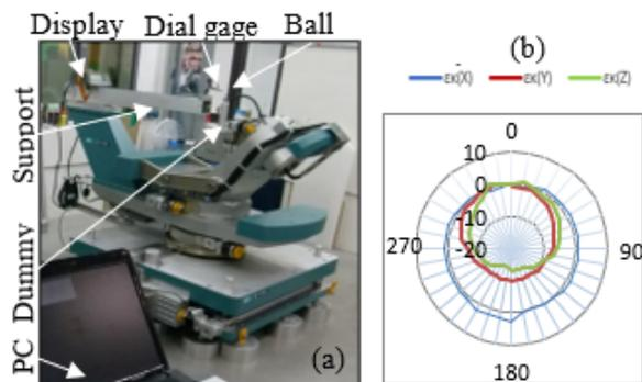
Figure 4: Measurements a) set-up and b) errors ( $\epsilon_{Xmax}$ =4 $\mu$ m,  $\epsilon_{Ymax}$ =10 $\mu$ m,  $\epsilon_{Zmax}$ =15 $\mu$ m,  $\kappa = \pm 180^\circ$ ).
