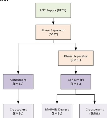
Figure 1: Cryogenics system: layered structure of hardware.
