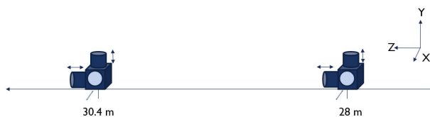
Figure 5: Placement of tri-axial accelerometers on the installation site with respect to the beam source.
