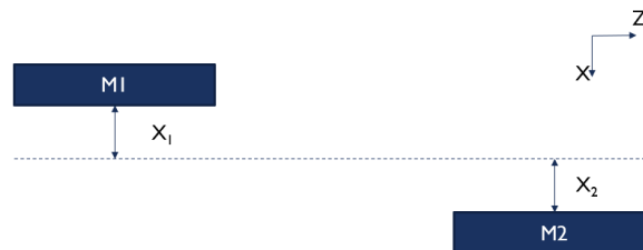
Figure 2: Top-down view of the mirror system showing absolute motion of each mirror with respect to the beam in the X direction.
