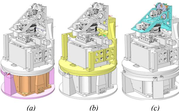
Figure 9: 3D model of the capacitive sensor metrology for scanning rotation stages (a) sample pitch stage metrology (b) linear sample scanning stages (c) sample yaw stage metrology.
