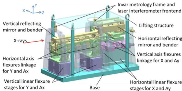
Figure 3: 3D model of the flexure stages system for K-B mirror alignment.
