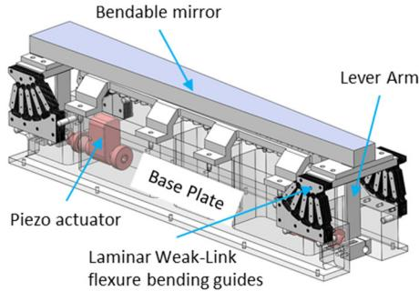
Figure 4: 3D model of KB mirror flexure bending mechanism.
