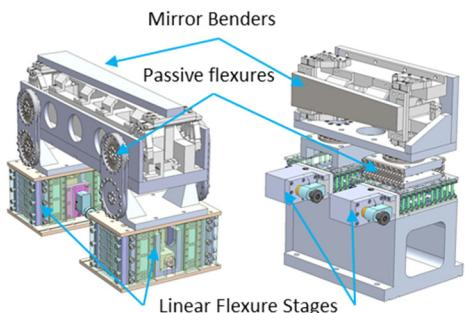
Figure 5: 3D model of horizontal and vertical KB alignment apparatuses.
