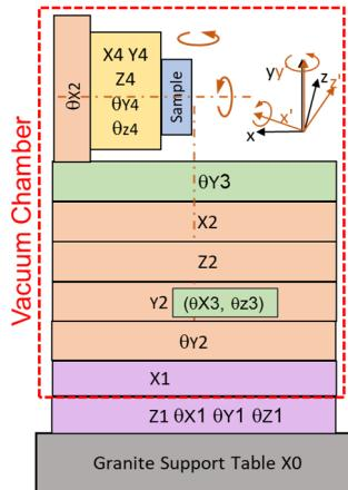
Figure 6: Schematic view of sample stages.
