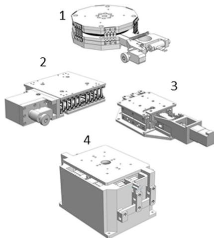
Figure 8: Custom flexure stages for sample scanning and sample.
