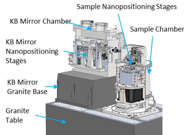
Figure 2: 3D model of the APS CSSI instrument.
