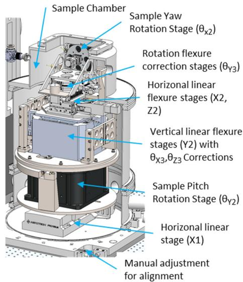
Figure 7: 3D model of the sample stages system.
