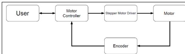
Figure 1: System architecture of Beamline Motor Control System.
