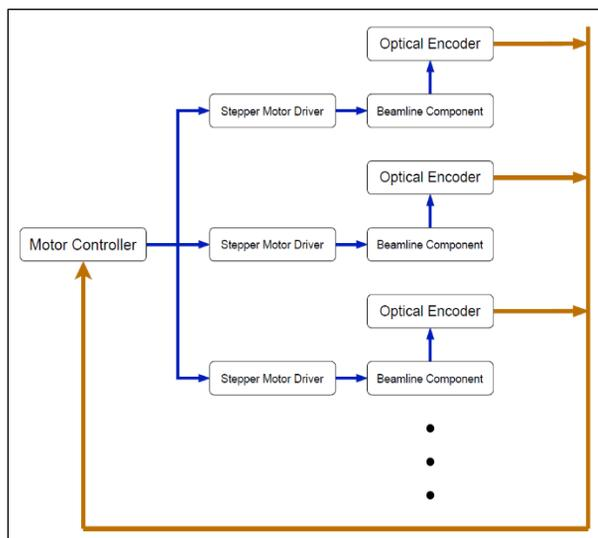
Figure 3: System architecture of Hardware.
