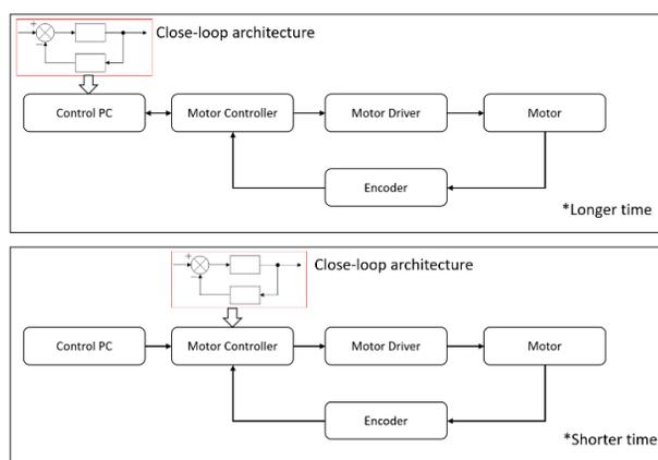
Figure 6: Close-loop diagram of software and firmware operation.
