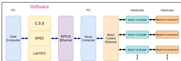
Figure 8: Software architecture diagram.
