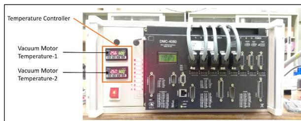
Figure 5: Temperature Controller & Motor Controller.
