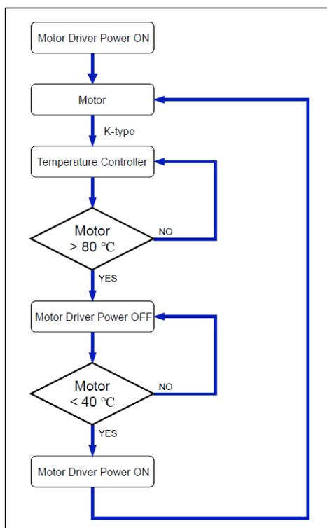
Figure 4: The temperature protection flow chart of the vacuum motor.
