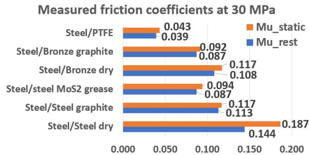
Figure 3: Measured friction coefficients at 30 MPa interface pressure for selected materials.
