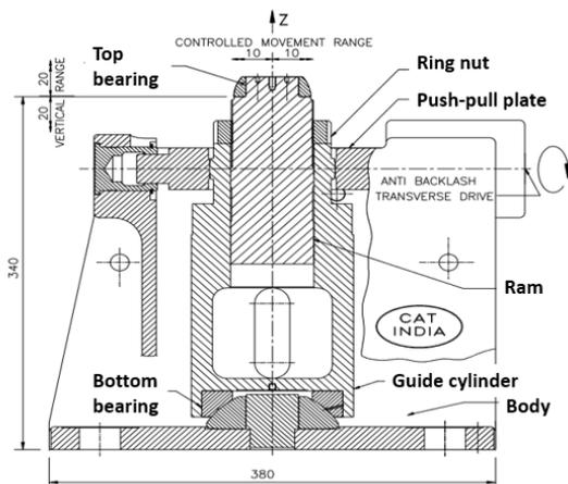
Figure 1: Transverse cross section of the LHC jack [2].
