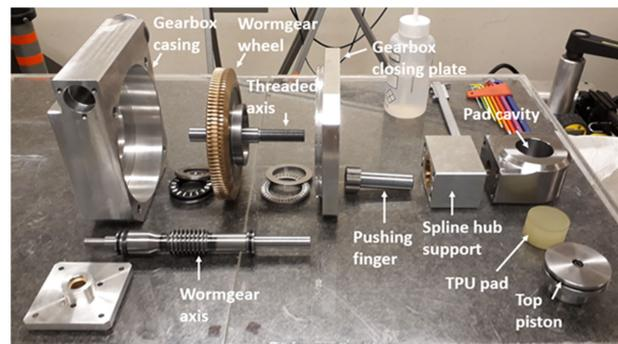
Figure 9: TPU pad prototype upon assembly.
