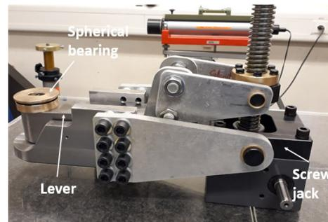
Figure 5: Prototype of the lifting lever design.
