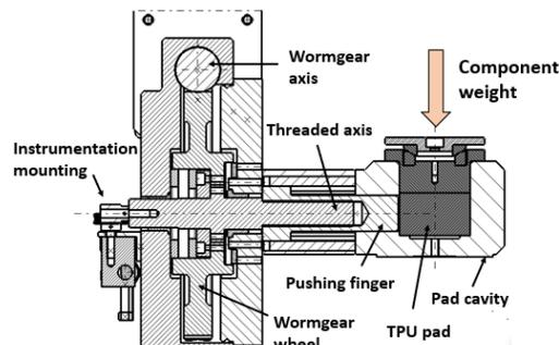
Figure 8: Cross-section of the prototype TPU pad design.
