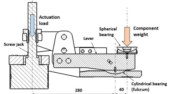
Figure 4: Cross section of the lifting lever solution.
