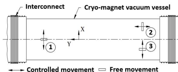
Figure 2: Top view of a cryomagnet - supporting jacks at position 1, 2 and 3 – adapted from [1].
