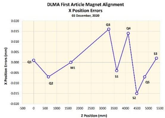
Figure 3: DLMA first article, magnet X-position errors.
