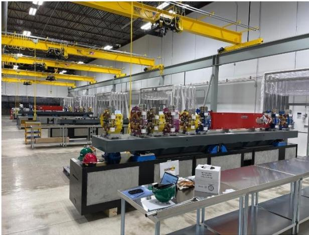
Figure 6: Picture showing the off-site Module Assembly Area including overhead cranes, retracted cleanrooms, and several modules in the magnet mounting process.
