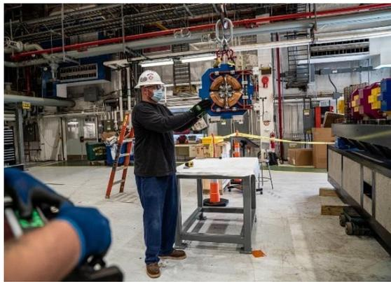
Figure 2: Quadrupole magnet enroute via overhead crane to its final location in the DLMA module (Image by JJ Starr/Argonne National Laboratory).
