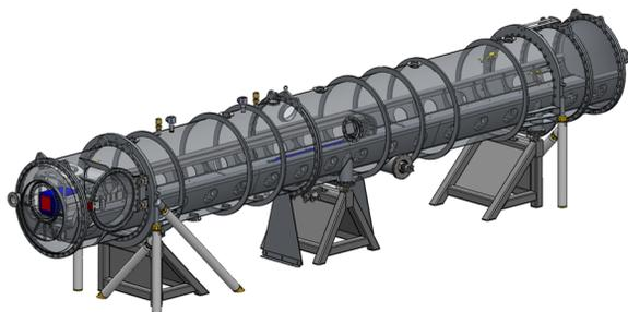
Figure 3: Flight Tube and SAXS detector.
