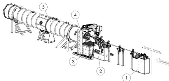
Figure 1: Main components of the endstation: (1) BCU I, (2) BCU II, (3) sample table, (4) detector gantry, and (5) flight tube.
