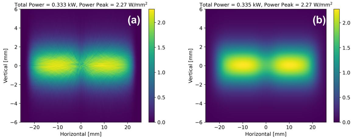
Figure 1: Power density distribution of ESRF-3PW: (a) Using ray-tracing and (b) New OASYS widget Wiggler Radiation.
