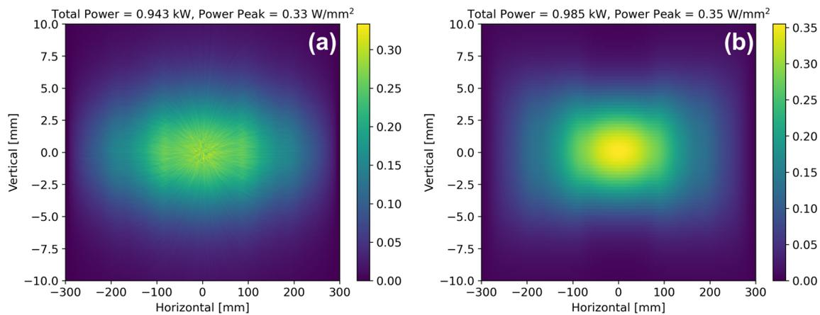
Figure 3: Power density distribution of BEATS project source: (a) Using ray-tracing and (b) New OASYS widget Wiggler Radiation.
