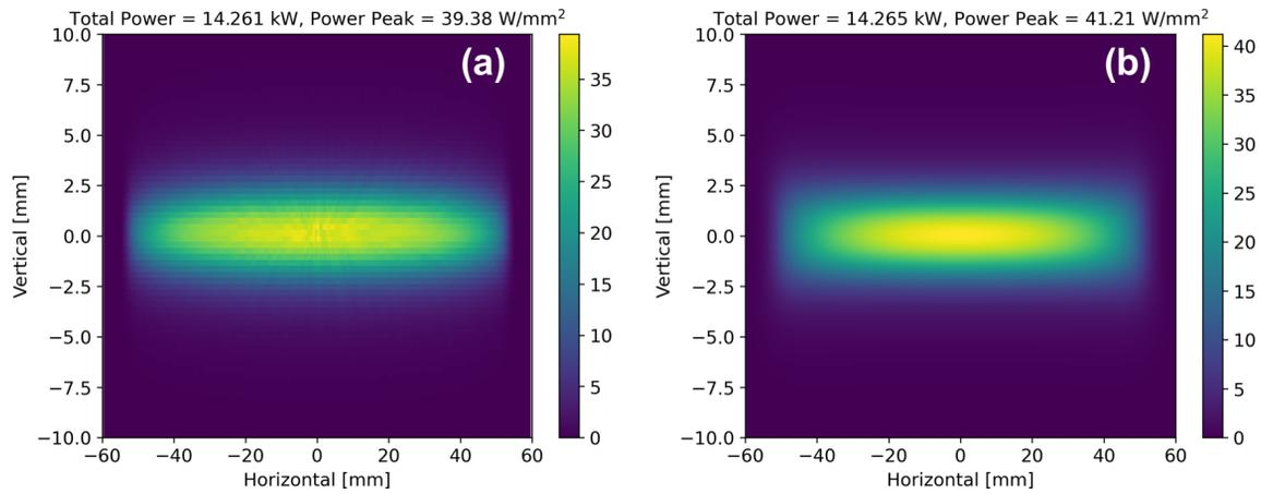
Figure 2: Power density distribution of ESRF-W150: (a) Using ray-tracing and (b) New OASYS widget Wiggler Radiation.
