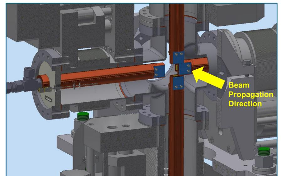
The SXBPM consists of four GaAs detector assemblies, each mounted on a copper heatsink. Two pairs of flange assemblies allow for the mounting of the detector assemblies to form vertical and horizontal pairs. The v-h configuration is shown above in which the vertical pair is positioned upstream of the horizontal pair. Reconfiguration to the h-v configuration can be done by removing and repositioning the flange assemblies.
