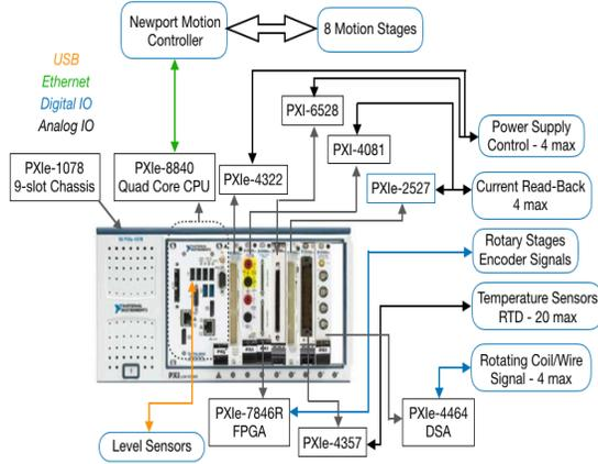
A National Instrument (NI) PXI system is employed for trigger generation and data acquisition (DAQ). The NI-PXI (PCI eXtensions for Instrumentation) is composed of three main hardware subsystems: a PXIe-1078 9-slot chassis, a PXIe-8840 embedded controller and seven plug-in modules.
