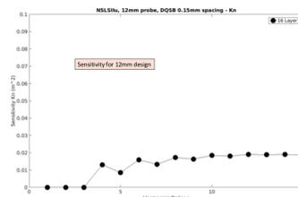
The coil will be suitable for measuring field quality to a level of 10 ppm of the main field (0.1 "units") up to the 15<sup>th</sup> harmonic with a sensitivity between 0.01 m<sup>2</sup> and 0.02 m<sup>2</sup> at the reference radius of 5 mm. The bucking factors are expected to be about 1000, therefore the DBuck signal should have a typical absolute measurement of the quadrupole field with an accuracy of about 0.15% (with no calibration).
