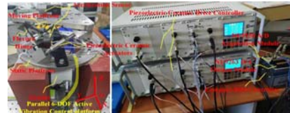
Figure 6: The active vibration control system base on parallel 6-DOF platform.
