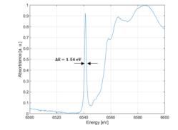
Figure 7: Beamline energy resolution measurement with KMNO<sub>4</sub> K edge.
