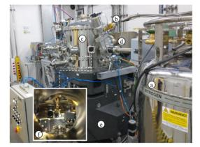
Figure 3: Photography of 4CM-CNB. Liquid nitrogen vessel (a), cryostat (b), vacuum chamber (c), ion pump (d), granite bench (e), and internal view (f).
