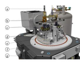
Figure 1: CAD representation of 4CM-CAT. Cryostat (a), copper straps (b), crystals (c), rotary stages (d), linear actuator module (e), vacuum chamber (f), granite bench (g).
