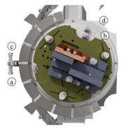
Figure 2: CAD representation of first channel-cut crystal module, containing the first (a) and second (b) diffraction surfaces and the crystal frame (c), which is clamped to the rotary stage (d) at three points 120° spaced.
