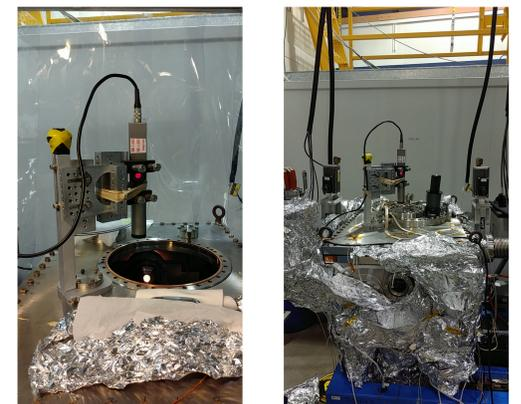
*In situ* autocollimator setup shown above and to the right was used to correlate XPS and autocollimator readings and verify that scan energy repeatability could be improved with in-vacuum scan angle encoding.
