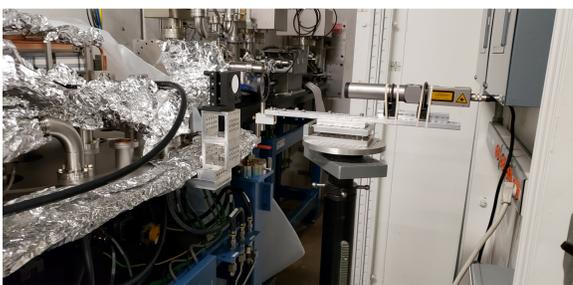
Autocollimator was aligned to upstream/inboard mirror at 2-ID prior to addition of reference mirror. Allowed verification of before/after repair of pitch and roll.
