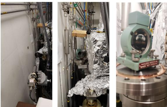
*In situ* autocollimator readings of both mirrors have been made under normal operating conditions utilizing viewports and a VLM in the case of downstream/outboard mirror which is inward facing.
