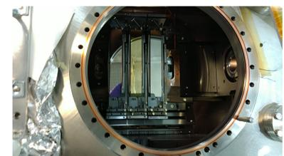
View thru open access port on 4-ID-C SGM showing third grating installed. Photo on bottom right shows how autocollimator was used to set new grating to have same pitch and roll as existing gratings.
