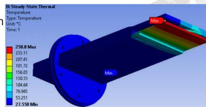
B:CA1 thermal analysis results assuming a scattered heat load
